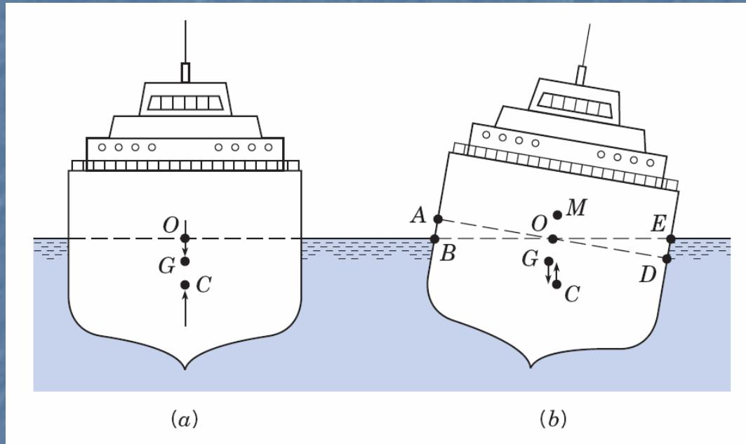
The point of intersection of the lines of action of the buoyant force before and after heel is called metacenter (M) and the distance (GM) is called the metacentric height
